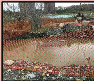
Water rose from below to fill the pit test holes.
